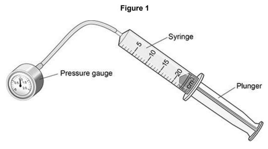
(a) When the plunger was pushed slowly into the syringe, the pressure in the syringe increased.
